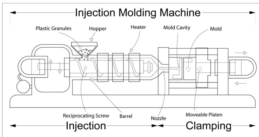
Figure 15: Injection Moulding
