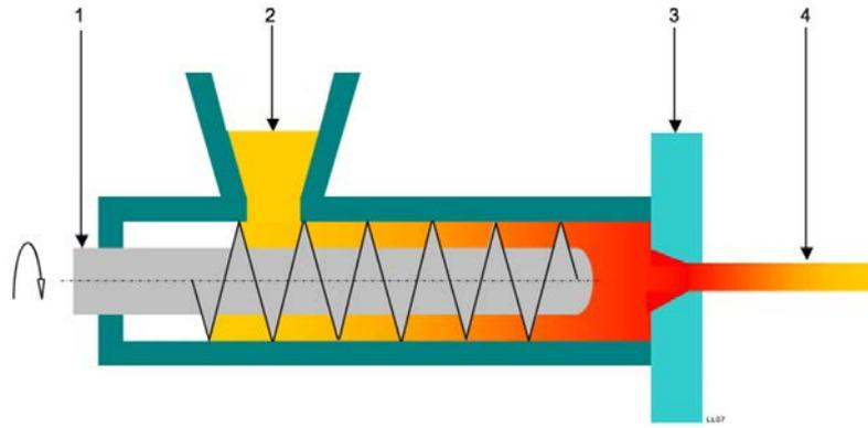
1 = Extruder, 2 = Plastic material, 3 = Extrusion die, 4 = Extrusion profile
